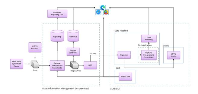
AVEVA Asset Information Management - hybrid is a standard driven information management solution comprised of the following on-premises components operated by the customer and cloud-hosted components operated by AVEVA. It is built from the following set of optional and mandatory elements:
