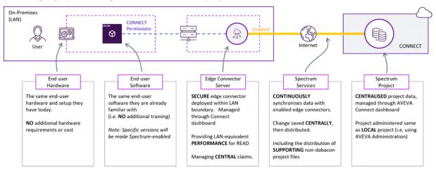
AVEVA Unified Engineering applications run on the user's desktop at their location, accessing databases and project data through Spectrum services running on the edge connector. When a user saves data, changes are written to cloud-hosted Spectrum storage by the client application, which in turn triggers the edge connector caches at all locations to be updated. Various other metadata services are also hosted in CONNECT.
