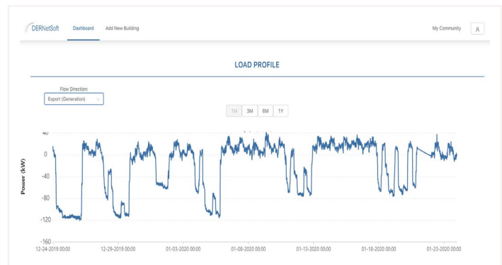
This dashboard shows energy production from fuel cells, indicating an excess of net metering on the weekends.
