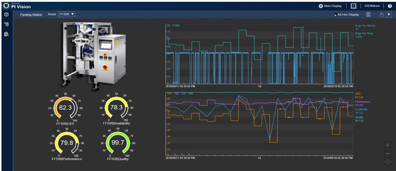
Illovo Sugar Africa uses PI Vision dashboards to see the real-time performance of 49 FFS machines across five sites in three countries.
